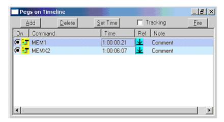
EMEMs, either Snapshots or Timelines, can be recalled and triggered using the PEGS dialog. Use MEM to recall but not run the EMEM. Use MEMX to recall and run.
