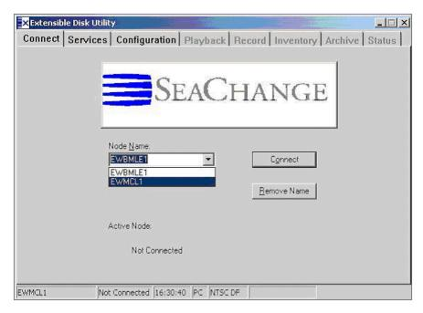
2 Select the MCL and the Configuration Tab and enable the VDCP Automation Protocol...
