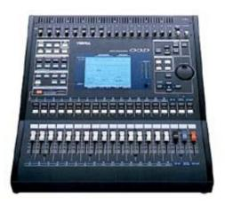
The Fastrack hybrid editing system interfaces to the 03D Serial Audio Mixer with a 6-pin DIN to 9-pin RS-422 serial control cable and Yamaha 03D midi-host serial protocol. Direct control of each individual fader and the learning of manual adjustments are possible.
